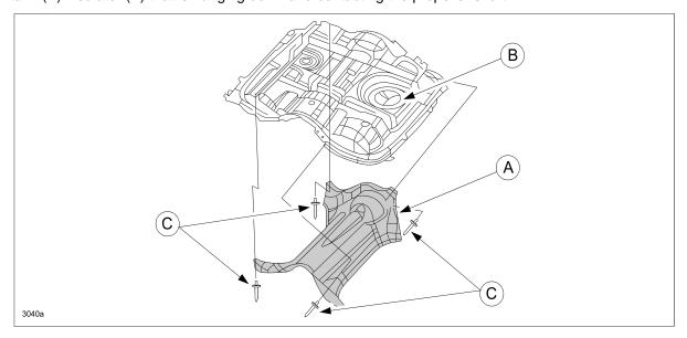
The rivets (C) may break when a load occurs. The rivet material has been changed to eliminate this concern. Customers having this concern should have their vehicle repaired using the following repair procedure.
