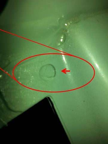
Tailgate lamp LH & RH water ingress - **potential root cause 2** Poorly fitted sealing patch to underside of tailgate upper in lamp recess
