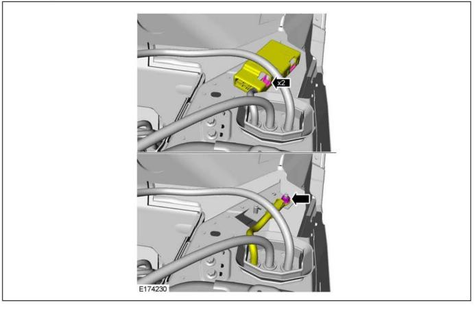
14. Remove battery cables from the vehicle body.
