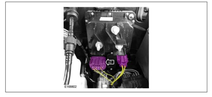
7. Remove the retaining nuts from the DBJB and remove from the mounting bracket.
