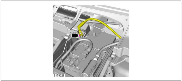
10. Disconnect the secondary battery positive connection and position the cable to one side.
