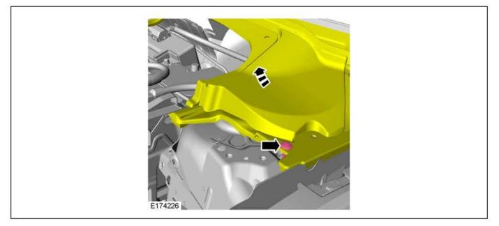
12. Disconnect the battery positive connection and position the cable to one side.
