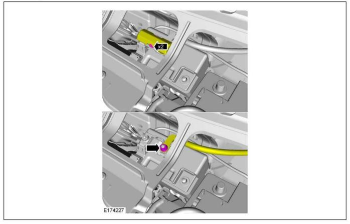
11. Remove the retaining clip and position the cowl panel to one side.
