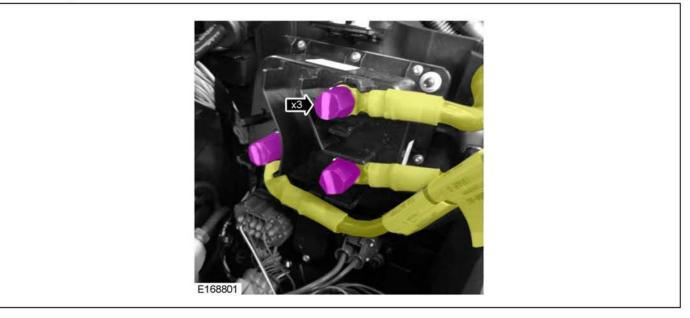
6. Disconnect the electrical connectors and position the electrical wiring harness to one side.
