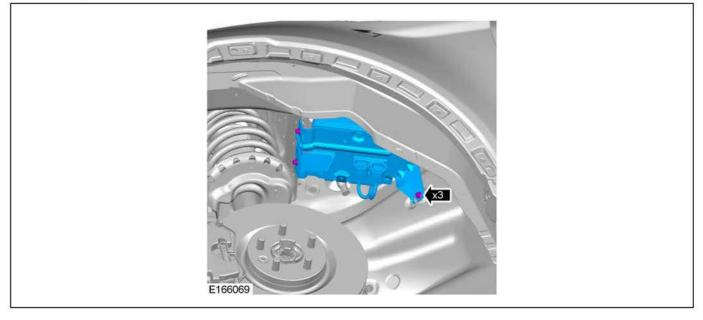
20. Disconnect the electrical connectors from the DBJB and position the electrical wiring harness to one side.
