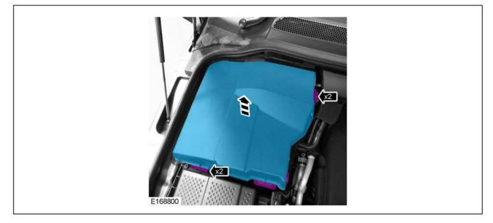
5. Remove the retaining nuts and position the electrical wiring to one side.
