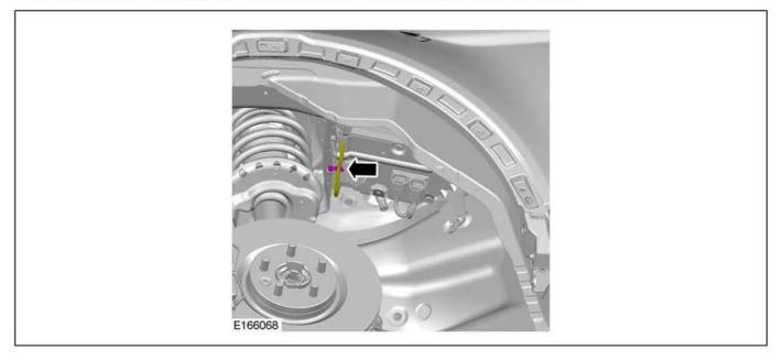
19. Remove the retaining bolts and the DBJB with mounting bracket.
