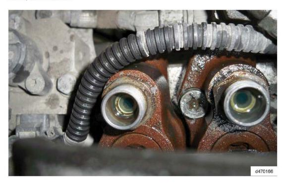
11. Clean the sealing area inside the high pressure fuel rail using a clean, lint-free cloth.
