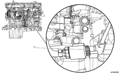
39. Using a zip tie (1), attach the fuel temperature wiring harness to the low pressure flange.
