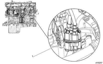
40. Install the chassis fuel feed and return lines on to the fuel filter module. Refer to OEM procedures.
