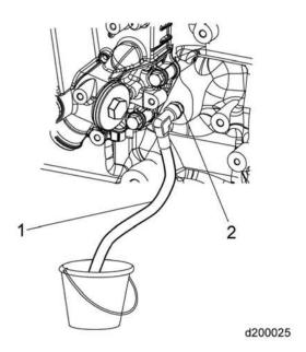
15. Close the drain plug. Torque to 30 N·m (22 lb·ft).
