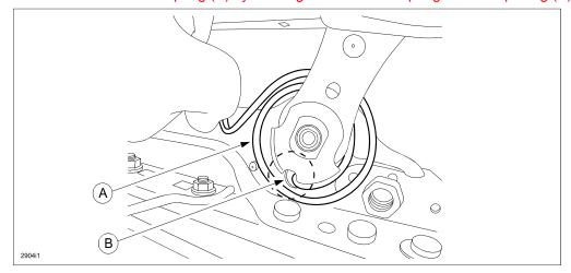
17. Hook the other end of the balance spring around the pin (A) using the hook tool (B) or with needle-nose pliers.
