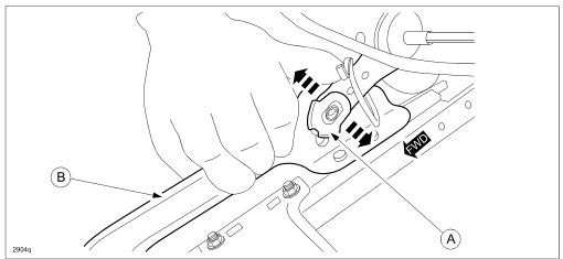
**NOTE:** Verify that the rear balance spring (A) has been properly positioned around the link (B). **CAUTION: DO NOT** damage the bushing during link installation.
