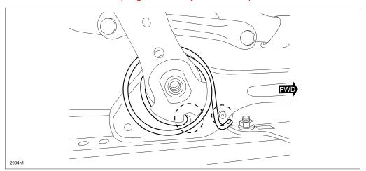
16. **INNER-SIDE:** Install the balance spring (A) by hooking the end of the spring into the opening (B).
