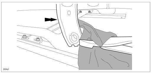
10. Tighten four (4) Torx T30 bolts to the specified torque.
