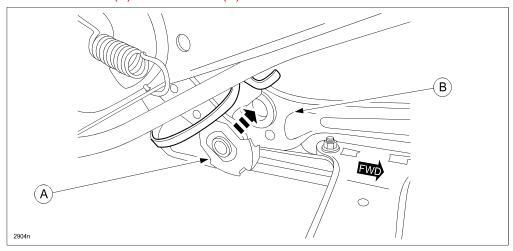
**CAUTION: DO NOT** damage the bushing during link installation.
