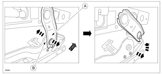
**NOTE:** Depending on specific production date of the vehicle, some CX-5 models may have plastic washers (A) installed between the front link (B) and the slider (C). **ALWAYS BE SURE TO RE-USE THE PLASTIC WASHERS** when installing the new seat adjuster lift unit.
