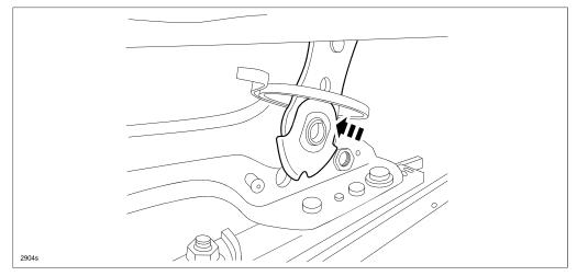
6. **Front-Outer:** Install the link (A) to the slider (B) while bending the slider inward and the link outward. **CAUTION: DO NOT** bend the slider too much as it may become deformed and cause improper operation.
