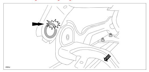
9. Install the link to the proper position using pliers and a shop rag.
