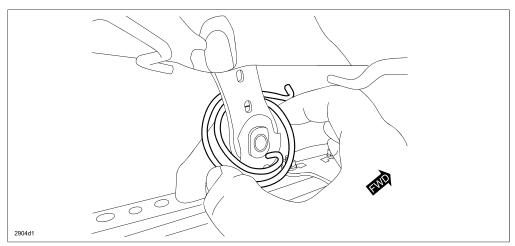
11. OUTER-SIDE: Install the balance spring (A) by hooking the end of the spring into the opening (B).
