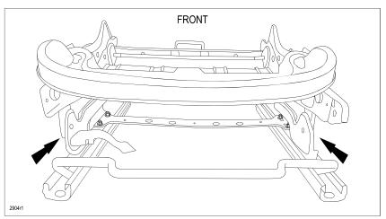
8. Detach the inner link (A) from the slider (B) by gently bending the slider outward and the link inward. **CAUTION: DO NOT** bend the slider too much as it may become deformed and cause improper operation.
