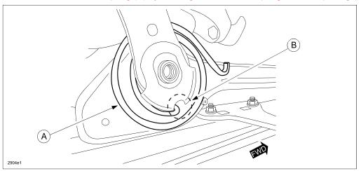
12. Hook the other end of the balance spring around the pin (A) using the hook tool (B) or with needle-nose pliers.
