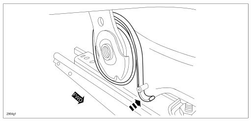
15. Verify that both ends of the balance spring are securely hooked into position.
