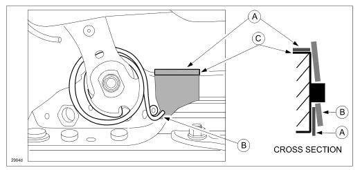
3. Using a flat-blade screwdriver with masking tape on the tip, gently pry the balance spring hook (A) away from the slider surface (B).
