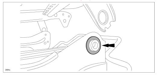
**CAUTION: DO NOT** damage the bushing during link installation.
