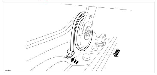
20. Verify that both ends of the balance spring are securely hooked into position.
