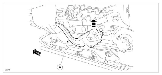
2. Starting with the **REAR** of the seat adjuster unit (as shown below), attach a piece of masking tape onto the inner sides of the left and right sliders to avoid scratch damage during the repair.
