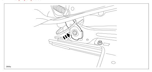
4. **Rear-Inner:** Install the link (A) onto the slider (B) while bending the slider outward and the link inward. **CAUTION: DO NOT** bend the slider too much as it may become deformed and cause improper operation.
