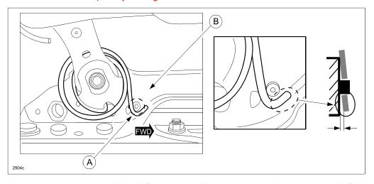
4. Release the rear balance spring (A) hook from the pin (B) using a tool with a hooked end (C) (as shown below) or with needle-nose pliers.
