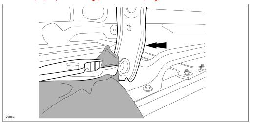
8. **Front-Inner:** Install the link (A) to the slider (B) while bending the slider inward and the link outward. **CAUTION: DO NOT** bend the slider too much as it may become deformed and cause improper operation.
