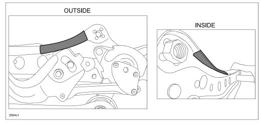
**NOTE:** When looking from the space between the seat cushion and the cover, the silver color of the seat lift frame is visible. By attaching the black tape to the upper frame, the silver color is covered up.
