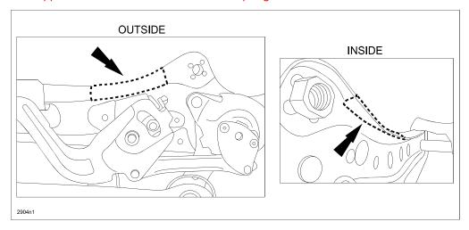
22. After degreasing the upper seat frame area, attach the piece of black tape (from kit) as shown below.
