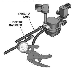
Watch the FTP sensor value on the HDS, apply vacuum until the value reads approximately 2.10V.
