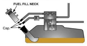
Watch the FTP sensor value on the HDS, and gently apply vacuum until the value reads approximately 2.10 V.
