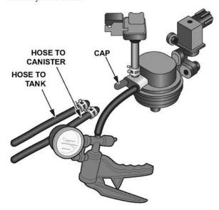
Watch the FTP sensor value on the HDS, gently apply vacuum until the value reads approximately 1.50 V (it takes very little vacuum to reach this value). Watch the value on the HDS for 20 seconds.
