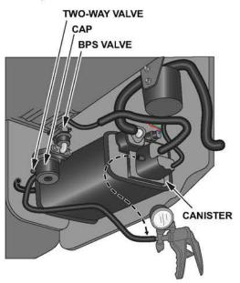
Watch the FTP sensor value on the HDS, gently apply vacuum until the value reads approximately 1.50 V (it takes very little vacuum to reach this value).
