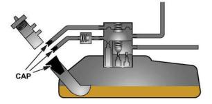
Watch the FTP sensor value on the HDS, apply vacuum until the value reads approximately 2.10 V.
