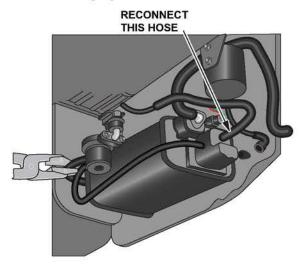
Disconnect the purge hose from the PCS valve that leads to the canister, and connect the vacuum pump.
