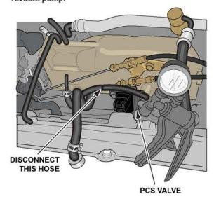
Enter the HDS PGM-FI menu, and select INSPECTION> EVAP TEST> MULTI SOLENOIDS. PCS ON> CVS ON> BPS ON.
