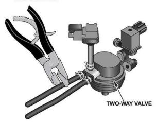
Disconnect the purge hose from the canister and connect a vacuum pump to the canister fitting.
