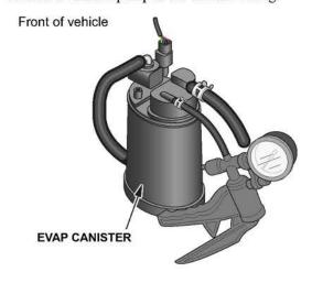
Enter the HDS PGM-FI menu, and select INSPECTION> EVAP TEST> MULTI SOLENOIDS> PCS ON> CVS ON> BPS ON.
