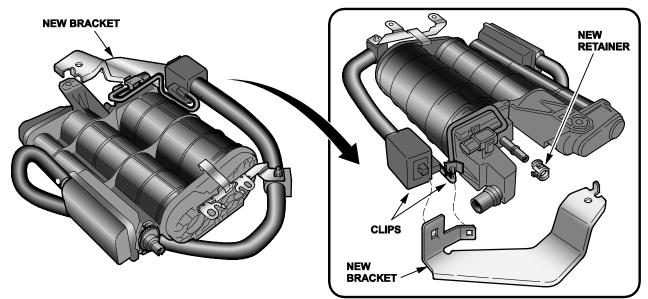
8. Reinstall the EVAP canister assembly and torque the bolts to 9.5 N·m (7 lb-ft).
