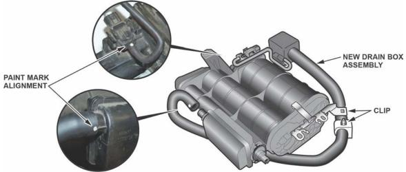
7. Install the new drain box bracket and new retainer as shown.
