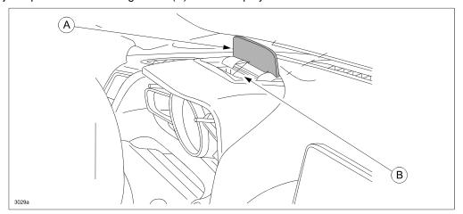
To correct the problem, the shape of the shaft and bearing part has been changed to increase the insertion force, thereby making the display harder to pop out of position.
