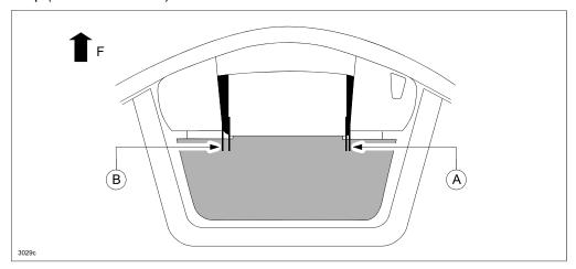
Replace the Active Driving Display (Heads Up Display) with a modified one according to the instructions on MS3 online or the Workshop Manual (section 09-10 ACTIVE DRIVING DISPLAY REMOVAL/INSTALLA-TION).
