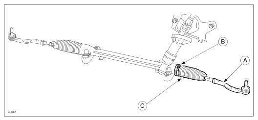
4. Insert a flathead screwdriver into the boot band (as shown below), then press the caulked area outward to remove the boot band.
