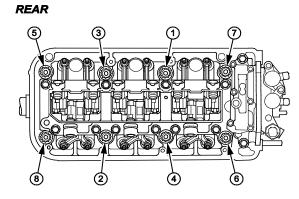
43. Measure the head bolts to determine if they need replacement. If either diameter is less than **11.3 mm (0.445 in)**, replace the cylinder head bolt.
