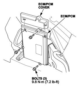
33. Remove the PCM connectors and harness clip. Remove the battery cables from the underhood fuse box.
