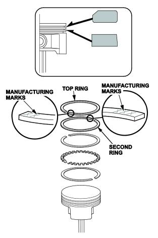
10. Position the ring end gaps as shown. NOTE: If the ring gaps are not positioned correctly, excessive blowby may occur.
