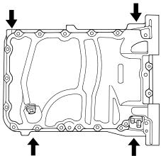
49. Remove the oil strainer and baffle plate.
