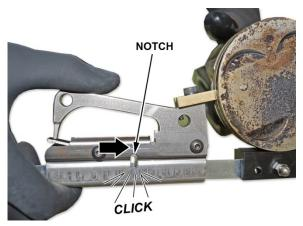
6. Hold the piston steady and rotate the tool counterclockwise five to six times to remove any carbon deposits in the piston ring grooves. **Do not** rotate the tool clockwise.
