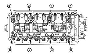
43. Measure the head bolts to determine if they need replacement. If either diameter is less than **11.3 mm (0.445 in)**, replace the cylinder head bolt.
