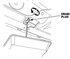
13. Install a 5/16th inner diameter rubber hose on the drain bolt at the rear of the engine block, loosen the drain bolt, and drain all remaining coolant. Then, disconnect the oil pressure switch connector.
