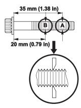
14. Apply new oil to the connecting rod bolt threads and flanges. Torque the bolts to **20 N•m (14 lb-ft)** then, tighten the connecting rod bolts an additional **90 degrees**.
