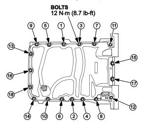
48. Using a flat-blade screwdriver, separate the oil pan from the engine block in the areas shown.
