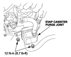
38. Remove the fuel rail connecting joint hose.
