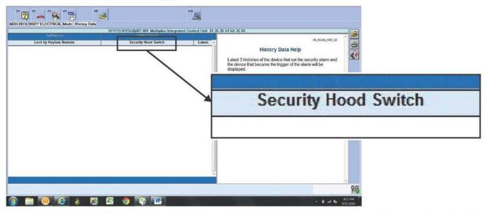
If the client complaint is "Security system will not arm", "Parking lights do not flash when setting security system", or "No feedback beep when pressing the lock button twice". Duplicate the complaint, then check the Body Electrical Data List using the HDS with the hood closed. If the Security Hood Switch signal reads ON (green) go to REPAIR PROCEDURE. If the Security Hood Switch OFF (red), this bulletin does not apply
