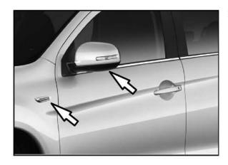
2015 Outlander Sport GT: Turn signals are relocated to the door mirrors from the front fender. A chrome garnish replaces the fender mounted lamp.
