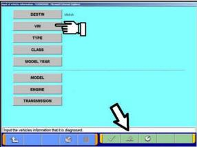
g. If the VIN or vehicle description displayed does not match the vehicle you are working on, click the eraser icon at the bottom of the page to erase vehicle data.
