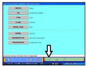
k. Confirm all data matches the vehicle and click the check mark at the bottom of the page.
