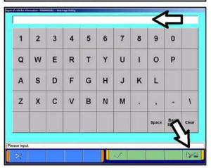
h. Click the icon in the lower RH corner of the screen to have MUT-III automatically read the VIN.
