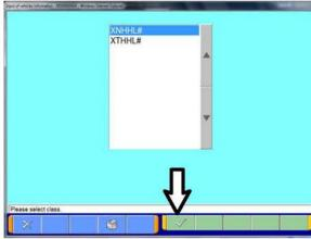
j. Look at the label on the passenger side B-pillar to identify the appropriate class. Select it and click the check mark at the bottom of the page.
