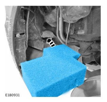
**5**Make sure the protective foam is installed in the correct area.
