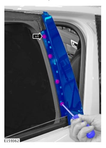
**11**Make sure the B-Pillar rear door exterior finisher is correctly located.
