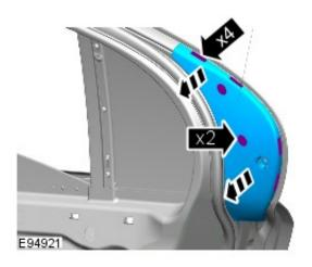
**5**Position to one side the rear door seal.
