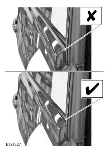
2Check the rear door exterior B-pillar finisher is correctly installed.
