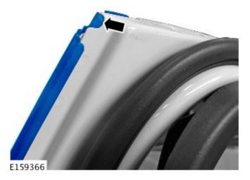
**12**Make sure the B-Pillar rear door exterior finisher is correctly located.
