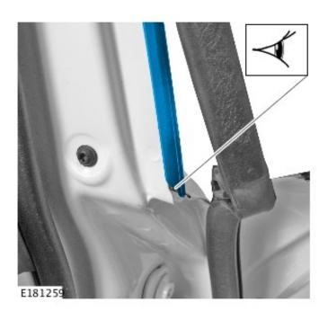
**3**Remove the rear door cap fixing cover and rear door cap fixing.
