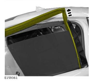
**9**Position to one side the rear door glass to gain access to the rear door B-Pillar fixings (see TOPIx Workshop Manual, Section 501-11).
