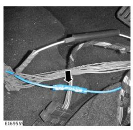
20. Tape the wiring harness using cloth tape.
