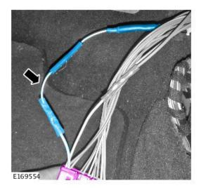
19. NOTE: Refer to the table above for wiring harness size and color in the harness repair kit.
