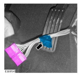
**10.** Open the four retention wings on the electrical connector C3BP01E.
