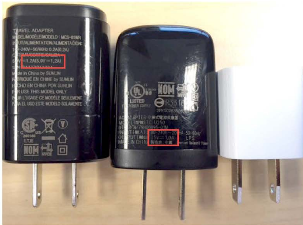
Figure 2. USB Smartphone charger with 1A current supply capability.
