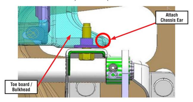
If the sound is confirmed to be originating from that location, use a small flat-blade screw driver to prevent movement of the upper layer while slightly separating it from the lower layer of the bracket as shown in the photo below. Operate the clutch pedal again and with the chassis ear in the same position as before, determine if the sound is changed or reduced while the screw driver is in place.
