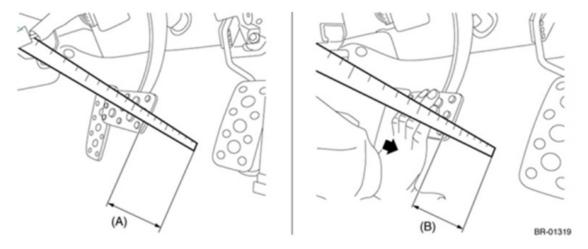
• The pedal stroke specification to activate the stop light switch is 5.5mm +/- 2.5mm (>3mm but <8mm).
