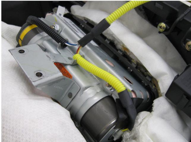
**STEP 14-** To eliminate a possible source of a rattling sound from the dash, wrap the 2 hooks and locator pin with non-woven material, p.n. SOA963W110 (or an equivalent self-adhesive foam) as shown below.
