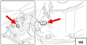
• The CVT fluid level is correct when it is up to bottom of the filler plug hole.
