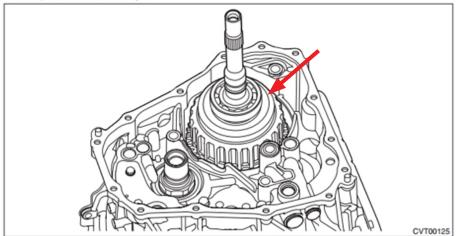
Measure the height "A" from the ST upper face to the ball bearing catch surface.
