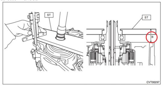
4) Obtain the thickness of reduction driven gear shim using the following formula to select zero to three reduction driven gear shims.
