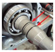
**IMPORTANT:** <u>BEFORE</u> applying any sealer to the cases, always trial fit them together to confirm proper spline alignment between the coupling sleeve, the drive motor input shaft and the primary pulley. The cases are too close together to facilitate turning the primary pulley retaining nut to get the splines aligned properly, especially when there is fresh sealer applied.
