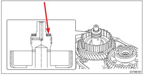
3) Using the ST, measure the height "A" from the ST end face to the thrust bearing catch surface of the transfer clutch assembly. ST 499575500 GAUGE
