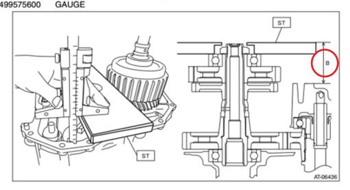
3) Obtain the thickness of transfer drive gear shim using the following formula to select one to three transfer drive gear shims.
