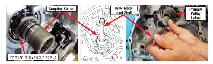
• Once proper spline alignment is confirmed, use some CVT fluid to hold the 6 o-rings in place between the cases during reassembly.
