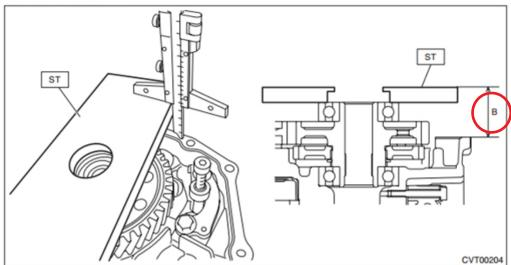
3) Obtain the thickness of transfer drive gear shim using the following formula to select zero to three transfer drive gear shims.
