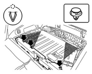
Remove the 3 retaining clips and release the claw securing the rear floor spacer then fold it over towards the front of the vehicle to expose the front edge of the stamped aluminum battery cover.
