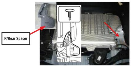
• CAREFULLY remove the right rear styrofoam floor spacer using a trim clip removal tool.
