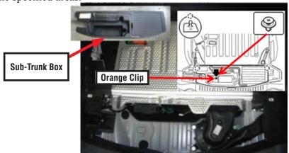
• Remove the rear floor and after releasing the orange retaining clip, remove the sub-trunk box.
