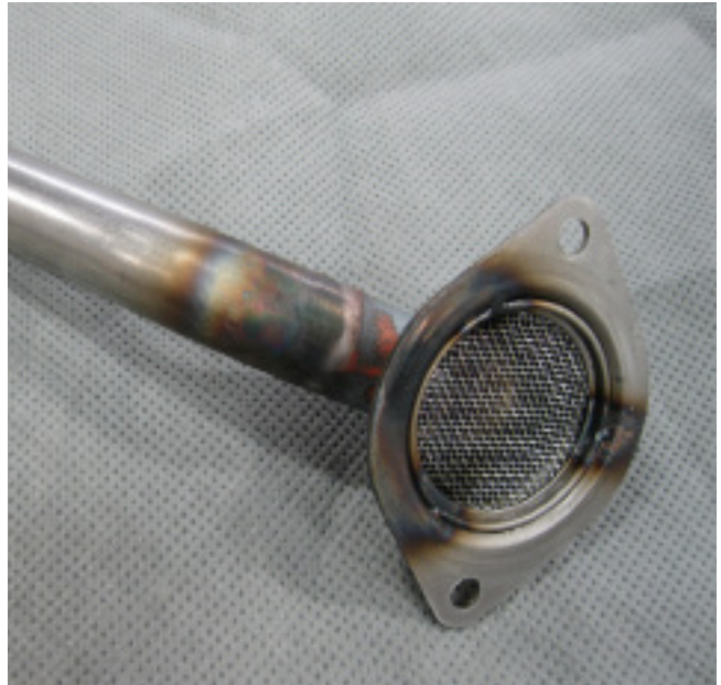
Oil Pick Up Tube/Filter Screen Assembly
