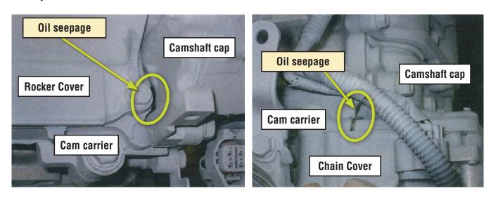
Apply Liquid Gasket, ThreeBond 1280B, (Part No. SOA5499100) or equivalent\* as shown below:
