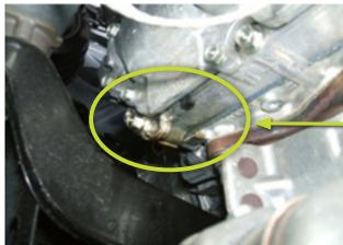
Cam carrier seepage seen from top left and lower right side of engine
