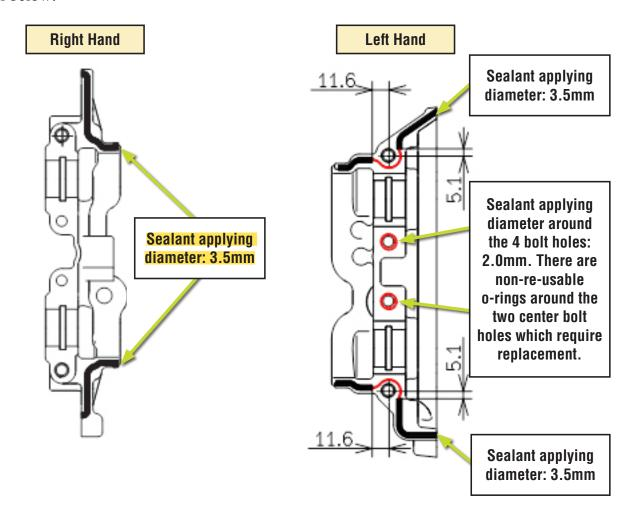
If you find engine oil seepage between the cylinder block and upper oil pan, remove the upper oil pan, clean the machined sealing surfaces thoroughly and then re-seal using Liquid Gasket ThreeBond 1280B, (Part No. SOA5499100) or equivalent\*. **Note:** The o-rings between the upper oil pan and the cylinder block along with those between the upper and lower oil pan will need to be replaced as they are not re-usable.
