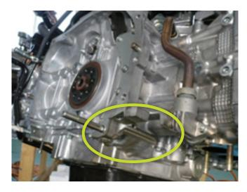
Photo shows seepage from upper oil pan to engine block sealing surfaces.
