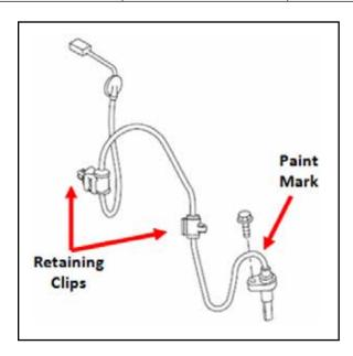
**NOTE:** The paint markings are located on the harness near the sensor mounting flange end.
