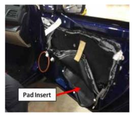
As shown in the illustrations below, remove the 2- 10mm hex bolts securing the door glass
