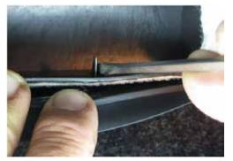
Using an electric drill with a 5/32" drill bit turning at **LOW SPEED**, **CAREFULLY** drill out the retaining rivets found between the "flaps" of the weatherstrip.
