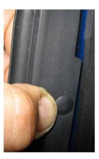
To complete this step, make sure the front of the weatherstrip is properly tucked in behind the chrome outer molding as shown below.
