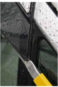
STEP 2 - Using a plastic trim tool under each end, CAREFULLY unseat the retaining clips and remove the outer door glass weatherstrip / chrome trim.
