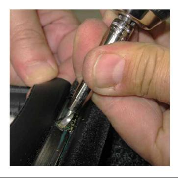
Fit the replacement inner weatherstrip to the trim panel. "Clamp" the new part to the door trim panel with your thumbs and fingers as shown below then bend the retaining claws over in the same direction as the originals (referenced earlier in this step) using your forefinger. The metal used for the backing and retaining claws of the weatherstrip is relatively pliable and easily bent into position.
