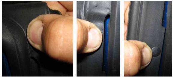
To complete the procedure, always make sure the front edge of the weatherstrip is properly tucked in behind the chrome outer molding as shown in the photos below.
