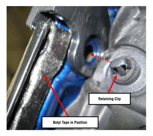
After the butyl tape is applied, refit the door frame weatherstrip and make sure the retaining clip "clips" back into the hole as shown to properly secure and position it. Work the weatherstrip onto the butyl tape with your thumbs making sure it is smooth and any bumps or high spots have been worked out.
