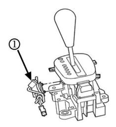
**Important:** For Ion models only, refer to *Diagnostic Starting Point - Automatic Transmission Shift Lock Control* and as necessary, *Shift Lock Control Solenoid (1) Replacement* in SI.
