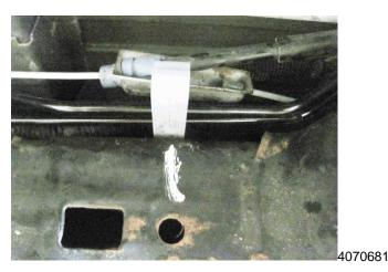
**Note:** Mark the location of the brake line mounting clip holes on the frame with a white marker to aid in the re-attachment of the brake line mounting clips.
