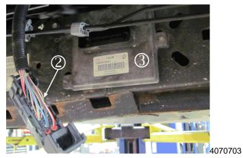
8. Disconnect the chassis wiring harness electrical connector (2) from the fuel pump flow control module (3).
