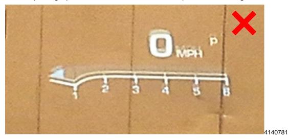
• If the front windshield displays a blurry HUD image, replace the front windshield. Proceed to step 2. The photograph with an 'X' is blurry and NOT an acceptable HUD image.
