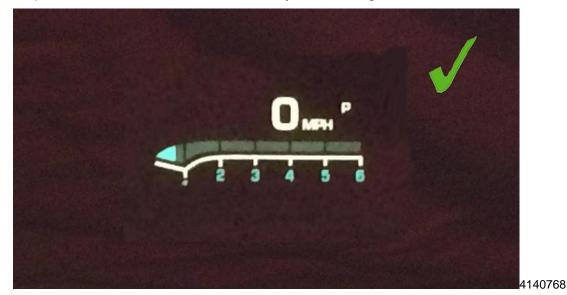
If the front windshield does NOT display a blurry HUD image, no further action is required. The photograph with a check mark is an acceptable HUD image.
