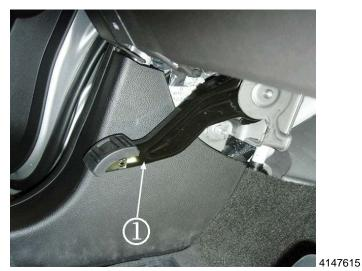
1. Locate the park brake pedal assembly (1). The park brake pedal assembly is located under the instrument panel on the driver side of the vehicle.
