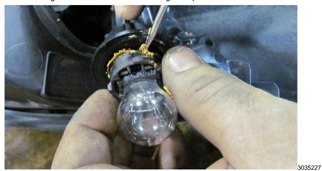
6. Clean old gasket material from the bulb socket.
