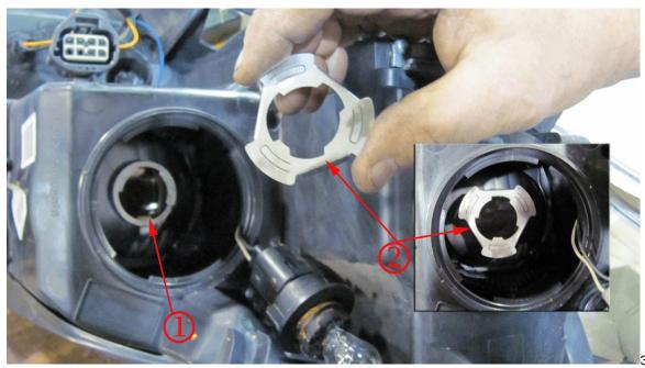
8. Align reinforcement plate tabs to the bulb reflector lugs (1). Install the reinforcement plate (2) onto the blub reflector (1) in the 12 o'clock position.
