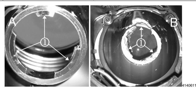
Note: Only replace the headlamp if the reflector lugs are damaged or missing.
