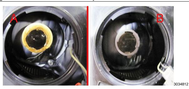
The "A" portion of the illustration shows the old gasket. The "B" portion of the illustration shows a clean bulb reflector.
