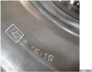
For torque converters built during the 2015 calendar year, inspect the first 3 digits of the Julian date, which are identified in the box, to determine if the torque converter must be replaced.
