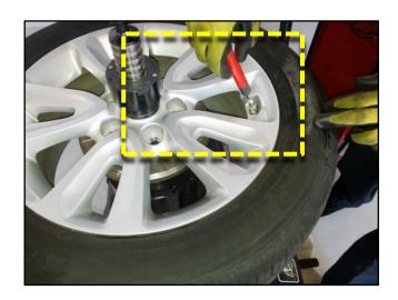
3. Use a ruler and yellow chalk to make reference marks 2" to either side of the valve stem, as shown
