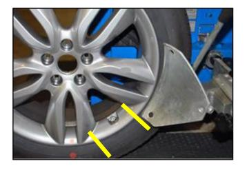
5. Use the machine's shoe to break the bead ONLY enough to expose the TPMS sensor. Then, remove the nut and pull the TPMS sensor from the wheel. NOTE: Be careful NOT to drop the TPMS sensor inside the wheel/tire assembly.
