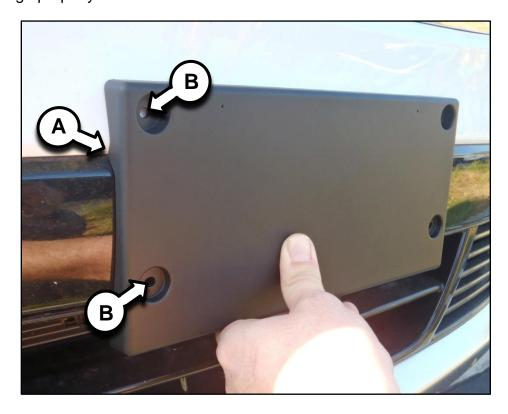
Incorrect fitment: P/N 86519 C6200 installed on a Sorento (UMa) EX or LX model. A= License plate holder profile does not match the curvature of the front fascia. B= Large gaps are evident
