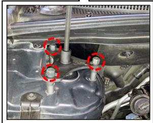
11. Lower the center bolt to compress the strut shaft.
