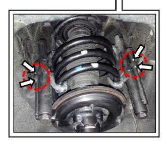
6. Use a white paint marker to create an alignment mark on the flat surface of the strut shaft, as shown.
