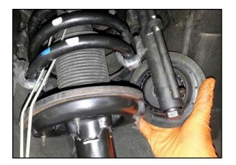
18. Lower the center bolt on the strut bearing remover tool and align it with the top of the strut shaft.
