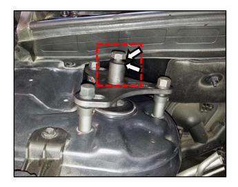
13. Locate the strut bearing remover cable and remove one side of the cable from the bracket.
