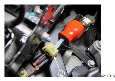
4. Remove the white lock clip (2) from the shift cable adjuster body using a flat blade screw driver.
