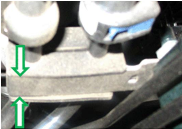
Bracket centered on rubber isolator.
