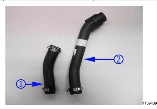
3.2 Match the new hose (2) to the original (1), aligning side by side.
