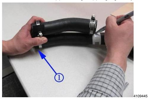
3.3 Using a paint pen or equivalent, mark the new hose to the original, starting with the notched fuel tank ends of the hoses so that both hoses are the same length.
