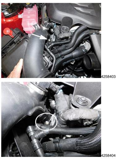
4. Loosen the engine harness bracket nut. DO NOT REMOVE.
