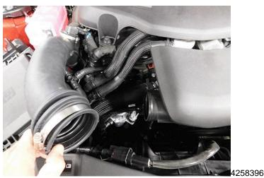
Note: Do not remove the intake snorkel from the turbo charger.
