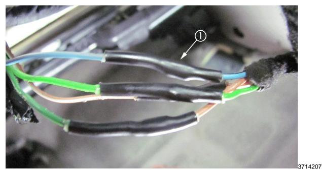
16. Center the heat shrink tube (1) over the splice and use the Ultratorch, part number J-38125-5, or another butane fueled soldering iron, to shrink and seal the heat shrink tube securely over the splice crimp and insulated wires.
