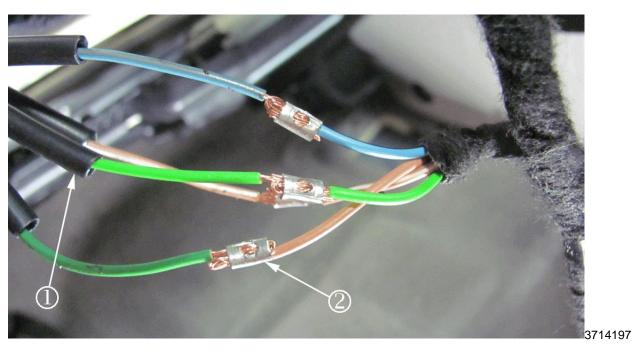
**Note**: Only use heat shrink tube, P/N 12355010, or an equivalent flexible adhesive-lined/moisture resistant heat shrink tube to perform the repair in this bulletin.
