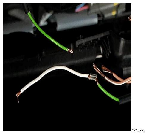
10. An additional wire clip and heat shrink tube will be required for each wire that needs to be lengthened.
