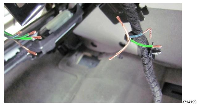
11. Remove 13 mm (1/2 in) of insulation from the seat and body harness wire ends.
