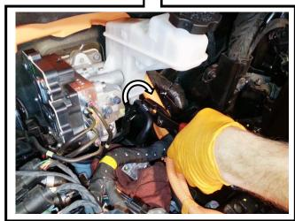
11. Prior to installation, inspect the Damping Chamber (L) to make sure the crush washer (M) is present.
