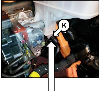
10. Use a pair of pliers to rotate the constant tension clamp 180° to the right.
