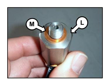
12. Install the Damping Chamber (N) onto the Master Cylinder (O), as shown.
