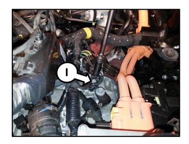
8. Lift the engine harness out of the way and remove the brake line (J), as shown.
