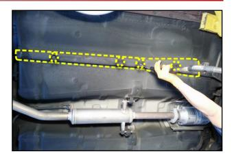
3. On Optima (MG) vehicles, use an air gun to remove debris or contaminants from the fuel tank straps, as shown.
