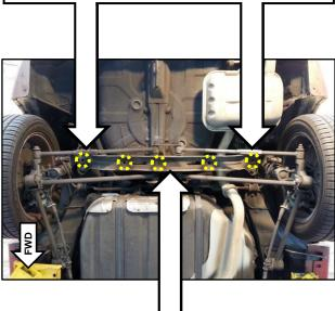
8. Remove any debris from the inside of the cross member using an air gun. NOTE: Make sure to insert the nozzle in multiple holes and rotate it in all directions to remove any foreign material or rust flakes.
