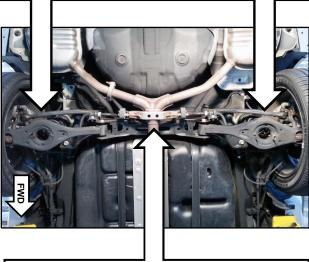
4. Apply undercoating onto the entire rear cross member, as shown. Do <u>NOT</u> apply undercoating to the exhaust pipe or other unrelated parts of the vehicle.
