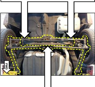
2. Use a metal bristle brush to clean and remove any rust scales or contaminants from all surfaces of the <u>rear cross</u> member.
