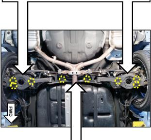
Remove any debris from the inside of the cross member using an air gun.
