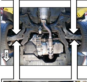
4. Remove any debris from the inside of each front lower control arm using an air gun. NOTE: make sure to insert the air gun in multiple holes and rotate it in all directions to completely remove any foreign material or rust flakes.
