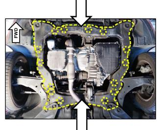
6. Remove any debris from the inside of the subframe using an air gun. NOTE: Make sure to insert the air gun in multiple holes and rotate it in all directions to remove any foreign material or rust flakes.
