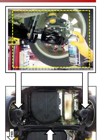
Apply undercoating onto the entire the torsion beam assembly, as shown.
