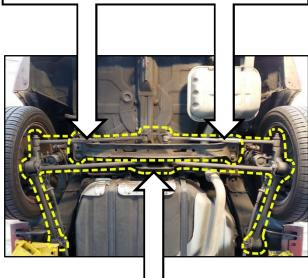
2. Apply undercoating onto the upper and lower surfaces of the cross member, as shown. Do <u>NOT</u> apply undercoating to the exhaust pipe or other unrelated parts of the vehicle.
