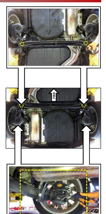
12. Use the air gun to remove any debris from the open ends of the torsion beam, spring perches, brake line mounts and shock mounts, as shown.
