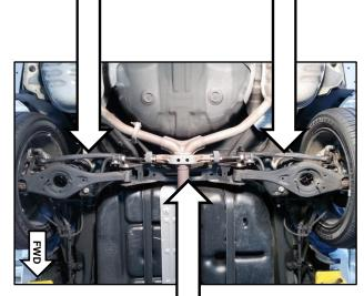
4. Use a metal bristle brush to clean and remove any rust scales or contaminants from all surfaces of the rear cross member.
