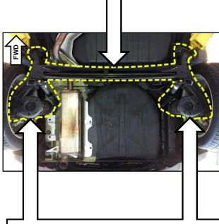
6. Use a metal bristle brush to clean and remove any rust scales or contaminants from the spring perches, brake line mounts and shock mounts, as shown.
