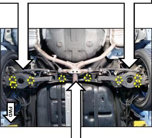
3. Apply cavity wax into every hole of the rear cross member, as shown. **NOTE:** make sure to vary the insertion angle of the nozzle to maximize coverage.
