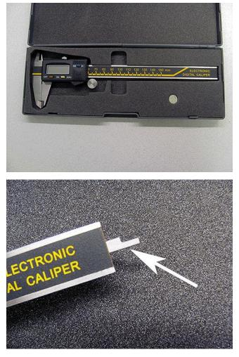
This inspection procedure requires the use of an electronic digital caliper with a depth measuring feature. Ensure the depth probe will fit into the gauge hole.
