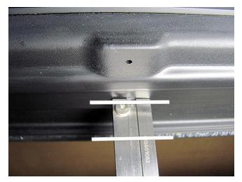
Ensure the base of the gauge is parallel to the edge of the panel.
