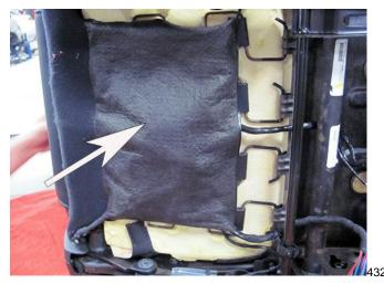
4. Remove the protective fabric as necessary.
