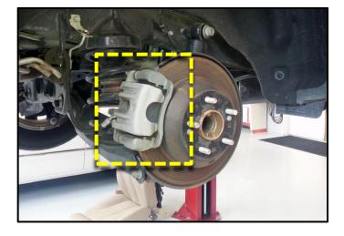
3. Remove the rear brake rotors.
