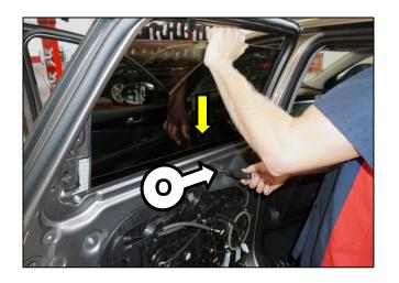
18. Remove one (1) screw (P) securing the window channel to the door, as shown.
