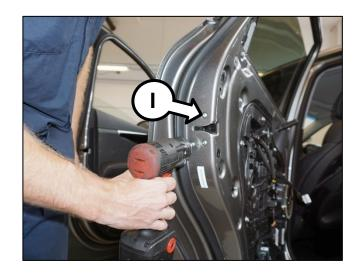
12. Remove the clear tape from the access hole (J) on the door and remove one (1) screw securing the door handle.
