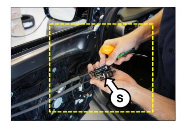
22. Remove the door module from the door, and guide the actuator cables and rubber boots (T) through the access holes in the door module, as shown.
