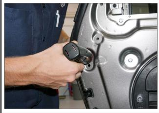
13. Pull the rear of the door handle (K) out and push the door handle forward to remove it from the door.
