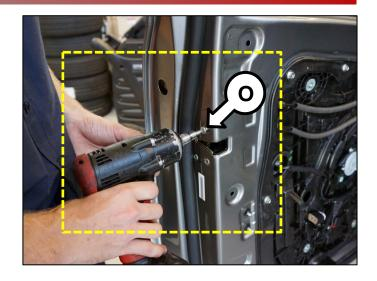
18. Remove two (2) bolts (P) securing the door glass to the regulator.
