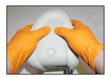
9. Verify the headrest trim piece is held securely in place. If the trim piece disengages, check and adjust the position of the clip (steps 6~7). Once the clip is properly adjusted, push the trim piece into position on the headrest. If the trim piece stays in place, proceed to step 10. If the trim piece disengages, replace the affected headrest with a new one.
