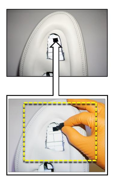
7. Push the clip forward until fully seated against the headrest body.
