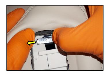
8. Push the sides of the headrest trim piece into the holes on the headrest, until firmly clipped in place.
