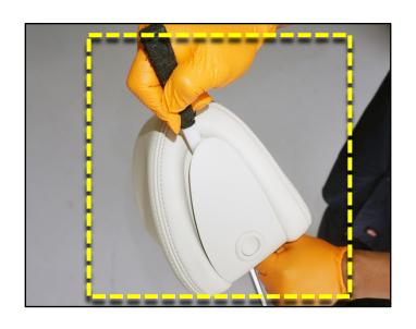
Carefully move the headrest trim piece out of the way and mark a set of "cut-lines" on either side of the headrest, as shown.
