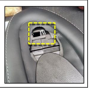
6. Insert the clip into the headrest, as shown.
